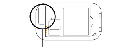
**Locate** the SSID label under the back cover
