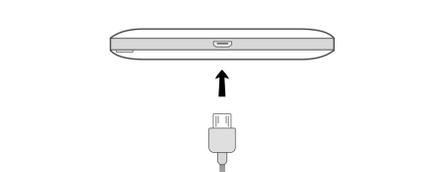
**Insert** the small USB connector into the charging port
