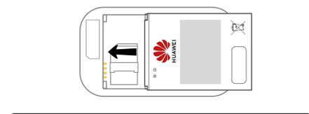
**Slide** the battery into place, aligning plus and minus symbols with gold prongs
