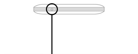
Turn the router on by pressing the power button
